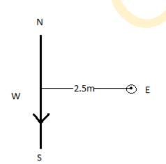
The current is going from the North to South direction in the horizontal plane and the point lies to the East of the wire. Applying Maxwell's right-hand thumb rule we can see that the direction of the magnetic field will be vertically upwards.
