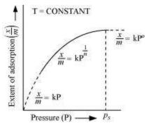
The plot between the extent of adsorption called the adsorption isotherm.
