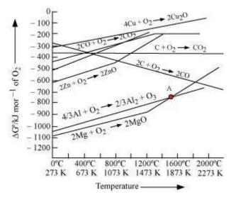
The above figure is a plot of Gibbs energy  $(\Delta G^{\circ})$  vs. T for formation of some oxides.
