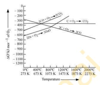
Reduction of ZnO to Zn is usually carried out at 1673 K. From the above figure, it can be observed that above 1073 K, the Gibbs free energy of formation of CO from C and above 1273 K, the Gibbs free energy of formation of CO<sub>2</sub> from C is lesser than the Gibbs free energy of formation of ZnO. Therefore, C can easily reduce ZnO to Zn.
